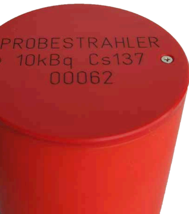
Fig. 5: Calibration source in Marinelli geometry (<10 kBq ^{137}\text{Cs} )
