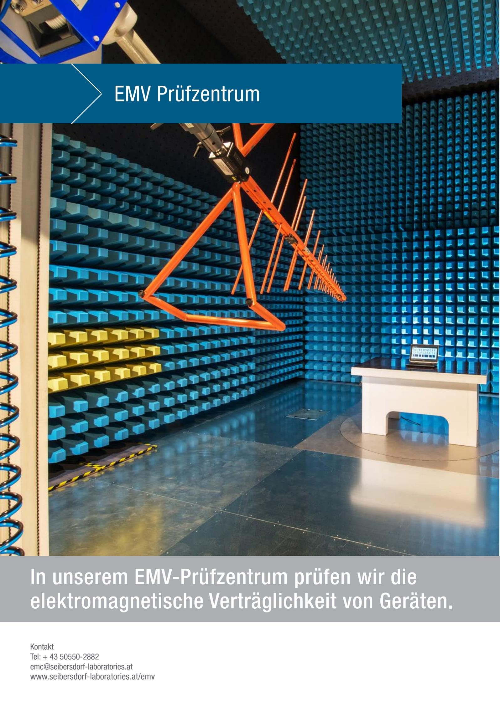
The image shows the interior of an EMV (Electromagnetic Compatibility) test chamber. The walls, floor, and ceiling are covered with blue and yellow pyramidal electromagnetic absorbers designed to eliminate reflections. A large orange robotic arm is suspended from the ceiling, holding a probe or antenna. In the foreground, there is a white control desk with a laptop on it. The lighting is focused on the center of the room.
