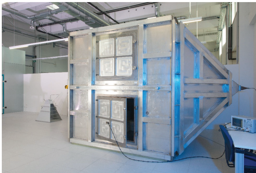
Figure 35: Large TEM cell for calibration of 60cm loop antennas
