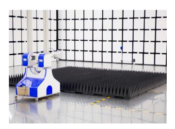
The EMC test site (Semi Anechoic Chamber, Fully Anechoic Room) of an accredited test house has to be **calibrated on a regular basis** (like all test instruments). It is a requirement of ISO 17025 to demonstrate the compliance of the test site at regular intervals - even when there was no modification in the construction since the last evaluation.
