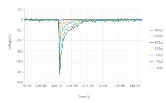
Single Event Transient (SET) waveforms of an electronic device encountered at different LETs realized by varying laser energies. Our SEE laser testing methodology provides invaluable insight into single event effects (SEE) and ensures robust system integrity for mission-critical applications.
