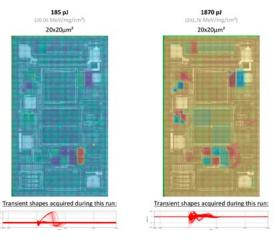
Single Event Effect Transient (SET) scan of an operational amplifier's full die, displaying transient amplitudes via a color map. Conducted with varied laser energies for low and high Linear Energy Transfer (LET), the assessment provides crucial insights into the device's radiation tolerance for enhanced system design.
