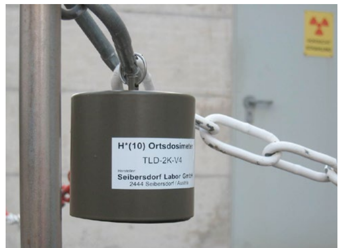
TLD-2K-V4 used for environmental monitoring
