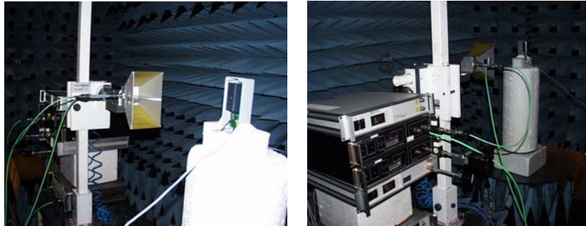
Radiated Susceptibility Test 1 – 18 GHz according to MIL-STD 461 D/E
