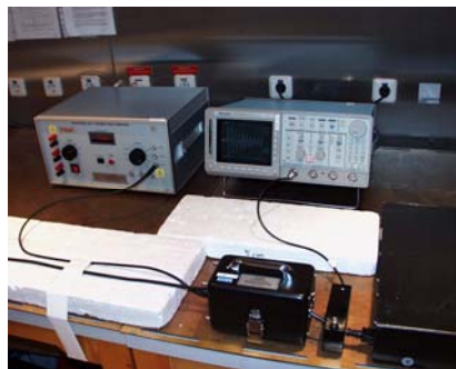
Bulk Cable Injection Test CS 116 according to MIL-STD 461
